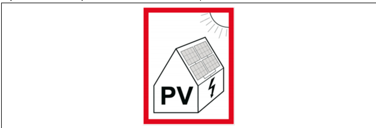
Figure 3.4 Example markings (signs) in Germany to identify the presence of PV systems 26
