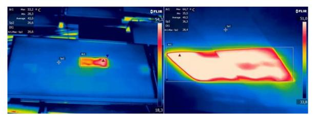
Figure 2-10: On the left side front view and on the right hand side rear side view of a PV module with overheated cell caused by internal cell problems.
