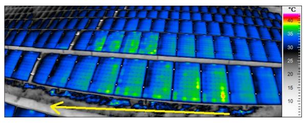
Figure 2-29: IRT image of a PID affected system under sunlight conditions. The modules in the foreground show PID patterns with warmer cells close to the bottom frame. The power
