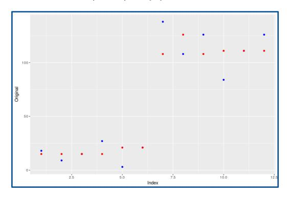
Figure 3-18: A simulated image edge represented as a 1-D vector (blue) and median filter of that vector (red).
