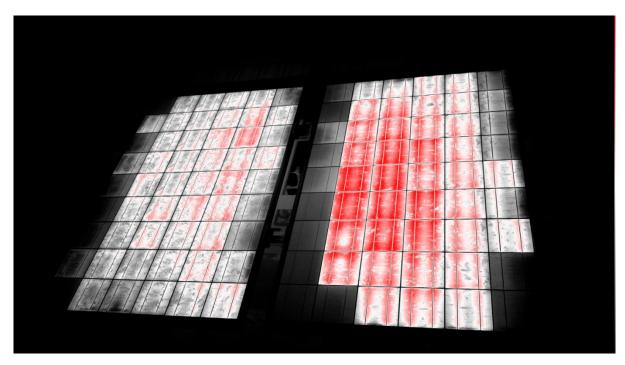
Figure 3-14: Night-time EL using a Consumer DSLR of PID affected modules, in a black-white-red colour scheme. The accumulated exposure time was around four minutes. The darkening of cell edge regions close to the frame can be observed, which is commonly attributed to current passing through the decreased parallel resistance instead of the PN-junction [82].
