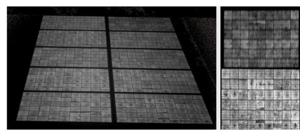
Figure 3-5: An outdoor EL performed with a consumer DSLR. The focus was performed on the front modules. Hence, as depicted to the right, only the front row can be imaged correctly, while one of the upper modules (right, top) is very blurry.
