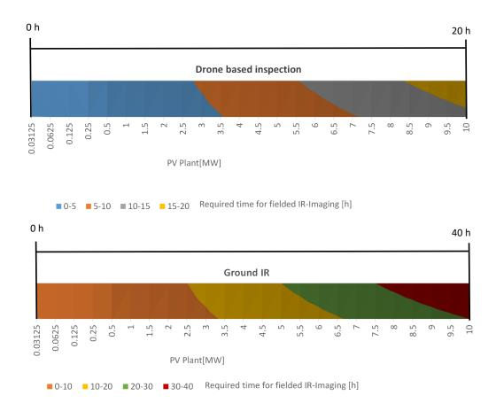
Figure 1-1 The required time for the inspection of PV modules using IR cameras, attached to a drone (top), and hand-held camera at the ground (bottom) with respect to the nominal power of the PV plant. The colours are used to identify the different time ranges for IR inspections.
