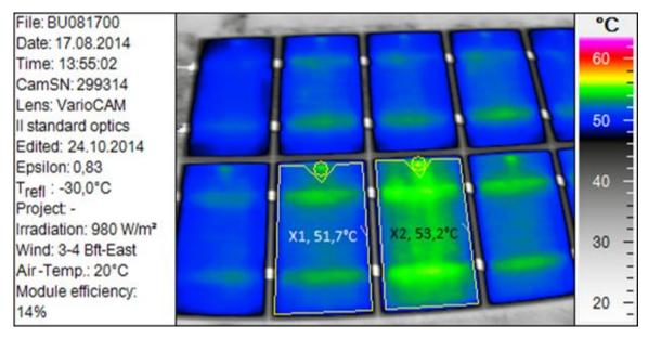
Figure 2-31: Example of plausibility check by determining the mean value of the temperature over the entire module excluding the junction box. In this example, the small temperature rise of 1.5 K was due to a different emissivity of the back sheet used for the two modules.
