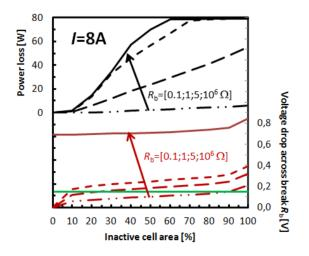
Figure 3-8: Simulated voltage drop across the break resistance of a separated cell part for a 230 Wp PV module at a forward current of 8 A (nominal current of the module). The green line marks 150 mV being able to detect with a low noise 12 bit CCD camera.
