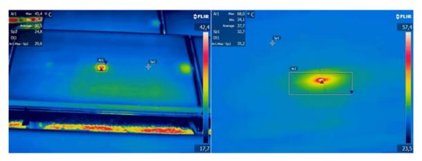
Figure 2-22: The left side IR image is derived from the front view of a PV module with heated cell interconnection. On the right hand side the rear side view of this heated cell interconnection is depicted.
