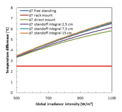
Figure 2-3: Example of temperature difference  $\Delta T$  calculated with Eq. (TDIFF) for a 15 % efficient PV module with  $T_{NOCT}$ =60 °C, an ambient temperature  $T_a$  of 20 °C, for various installation situations and no wind having an active and an inactive part of the module. The red line represents a minimum temperature difference needed to assure that it is not an artificial effect.
