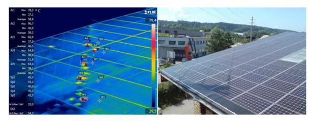
Figure 2-15: PV module shows overheated cells due to shading by the medium voltage overhead lines and its pylon.
