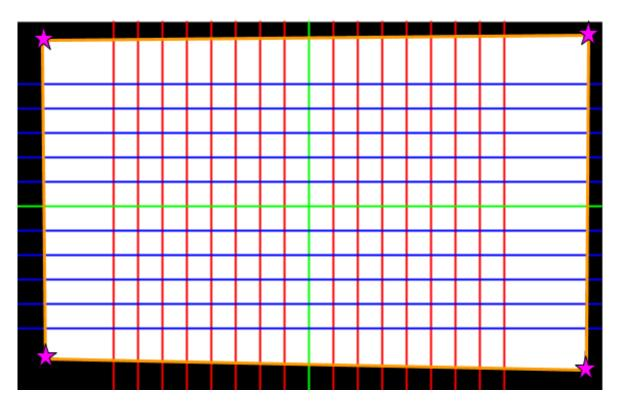
Figure 3-23: Visualization of the steps used to identify the four corners of the active cell region. The green lines are references lines for the mid-points in the x and y dimensions. Blue lines indicate horizontal vector slices. Red lines indicate vertical vector slices. Orange lines represent linear regression fits of the active area edges. Magenta stars represent the four corners of the active cell regions where the linear regression fits intersect.
