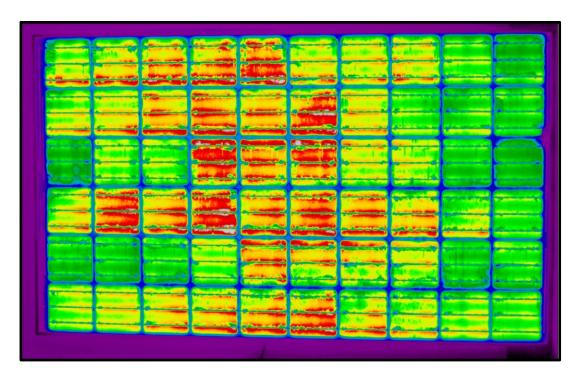
Figure 3-20: A median filtered grayscale EL image. Displayed using a spectral colour mapping.
