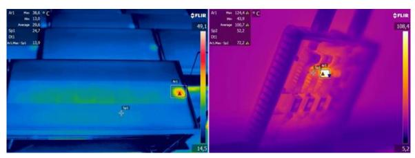
Figure 2-17: On the left side, front view PV module with overheated junction box and on the right hand side, rear side view with open junction box and overheated diode.
