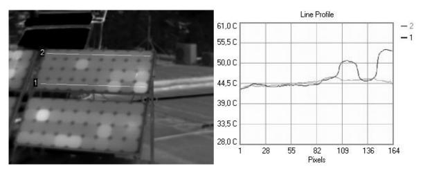
Figure 2-1: Example of a simple analysis based on temperature line profiles of ROIs corresponding to hot spots in a PV module under short circuit conditions.
