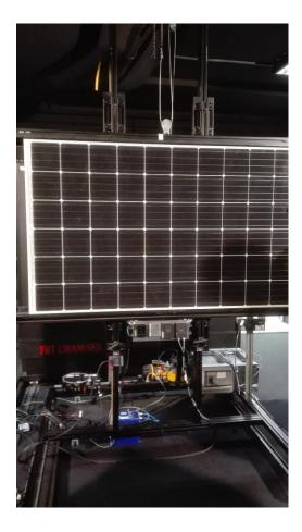
Figure 3-1: Photo of a typical experimental setup for EL tests in the laboratory, taken in the PV lab at SUPSI, Lugano, Switzerland.
