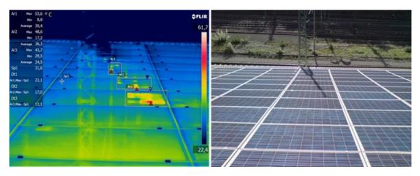
Figure 2-13: PV Module shows overheated cells due to shading by metal rod.
