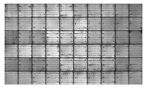
Figure 3-24: A perspective transformed EL image into a uniform orientation using the four corner points represented by the magenta stars in Figure 3-23.
