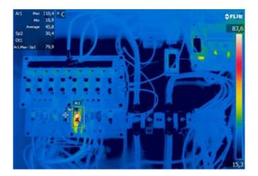
Figure 2-23: DC combiner box with overheated string fuse/spring clamp connection.
