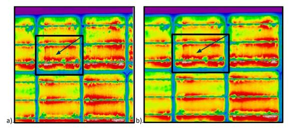
Figure 3-19: An EL image section displayed using a coloured spectral mapping for ease of visualization. The arrow points to a bright pixel value that was reduced by filtering.
