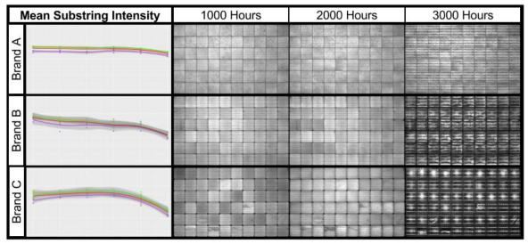
Figure 3-25: Mean substring intensity for three brands of modules over 3000 hours of dampheat exposure [90]. The plots show 500, 1000, 1500, 2000, 2500, and 3000 hour steps of exposure along the x-axis, however, for only the corresponding 1000, 2000, and 3000 hour steps are shown as EL images. At each time-step, data points for 3 samples are plotted. The standard error is shown as a gray bounding shadow behind the data points.
