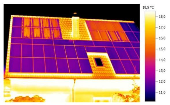
Figure 2-30: IRT image of a PID-s affected rooftop system with applied current during the night. In this case, the cooler cells are the PID-s affected cells [58].
