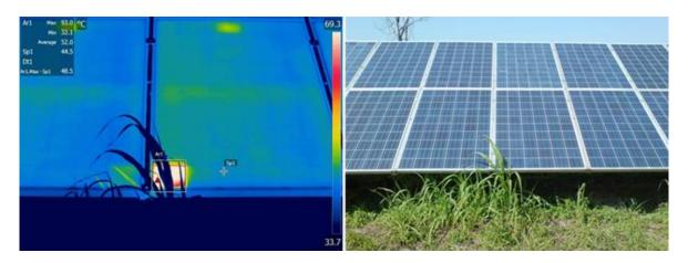
Figure 2-14: PV module shows overheated cells due to shading by plants.
