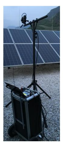
Figure 3-6: GreatEyes LumiSolar outdoor measurement system for field tests of PV modules.
