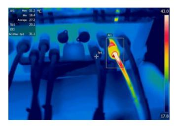
Figure 2-24: String inverter with overheated DC connector.
