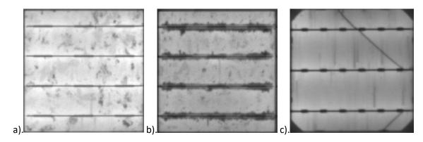
Figure 3-27: Characteristic cells for each of the 3 cell types classified a). Good/clean, b). Busbar corroded and c). Cracked.
