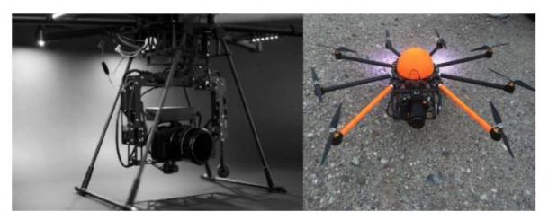
Figure 3-7: EL camera mounted on octocopter [79].
