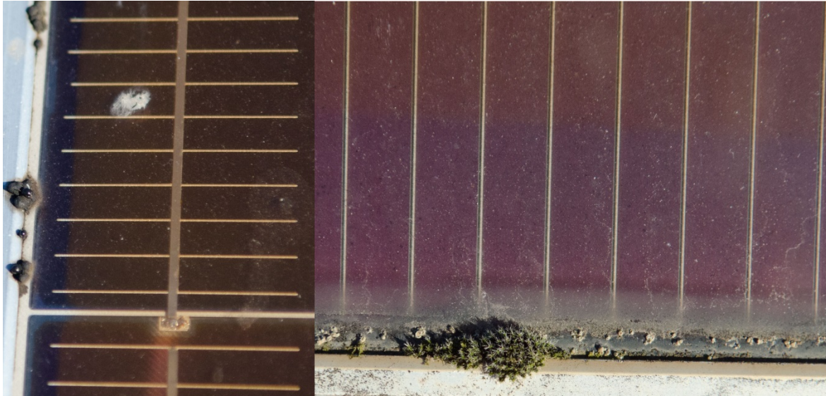
Fig. 38: Example of bird droppings (left) and moss (right) on a PV module.
