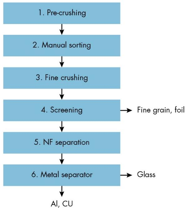
*Figure 2. Schematic drawing of c-Si module recycling process used by Respondent #2. All output products are further treated by other external specialized waste-treatment companies or are put in a landfill. Note that there is not a separate process step for frame separation.*
