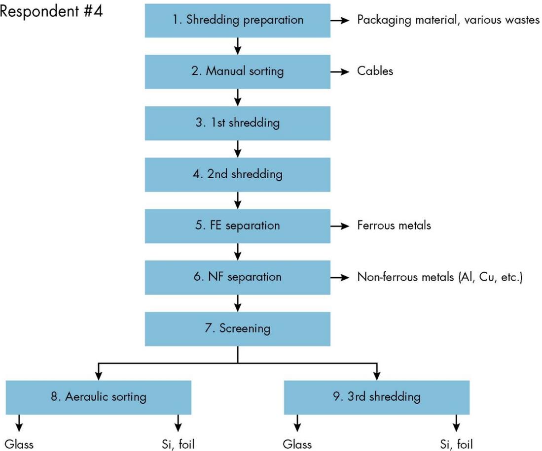
Figure 4. Schematic recycling process at Nike S.r.l.
