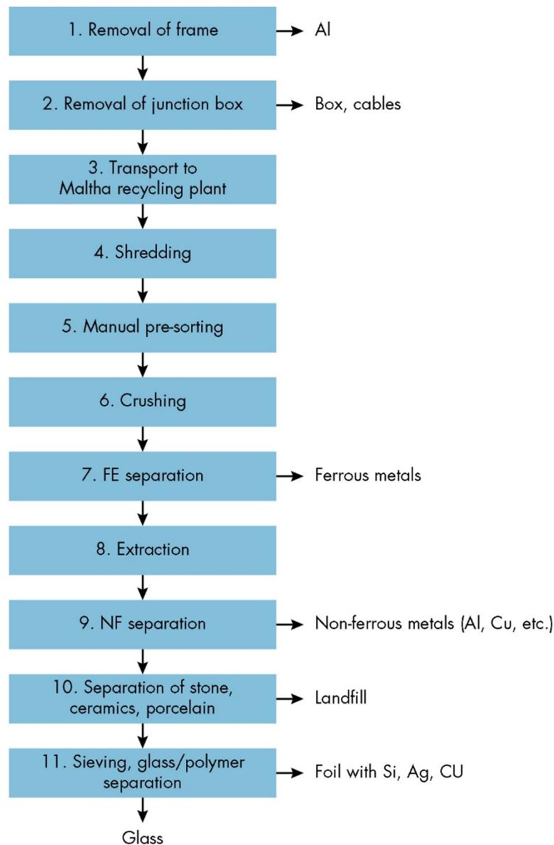
Figure 3. Schematic recycling process of Respondent #3. Note that transport to Maltha is not included in the LCI data for this respondent.
