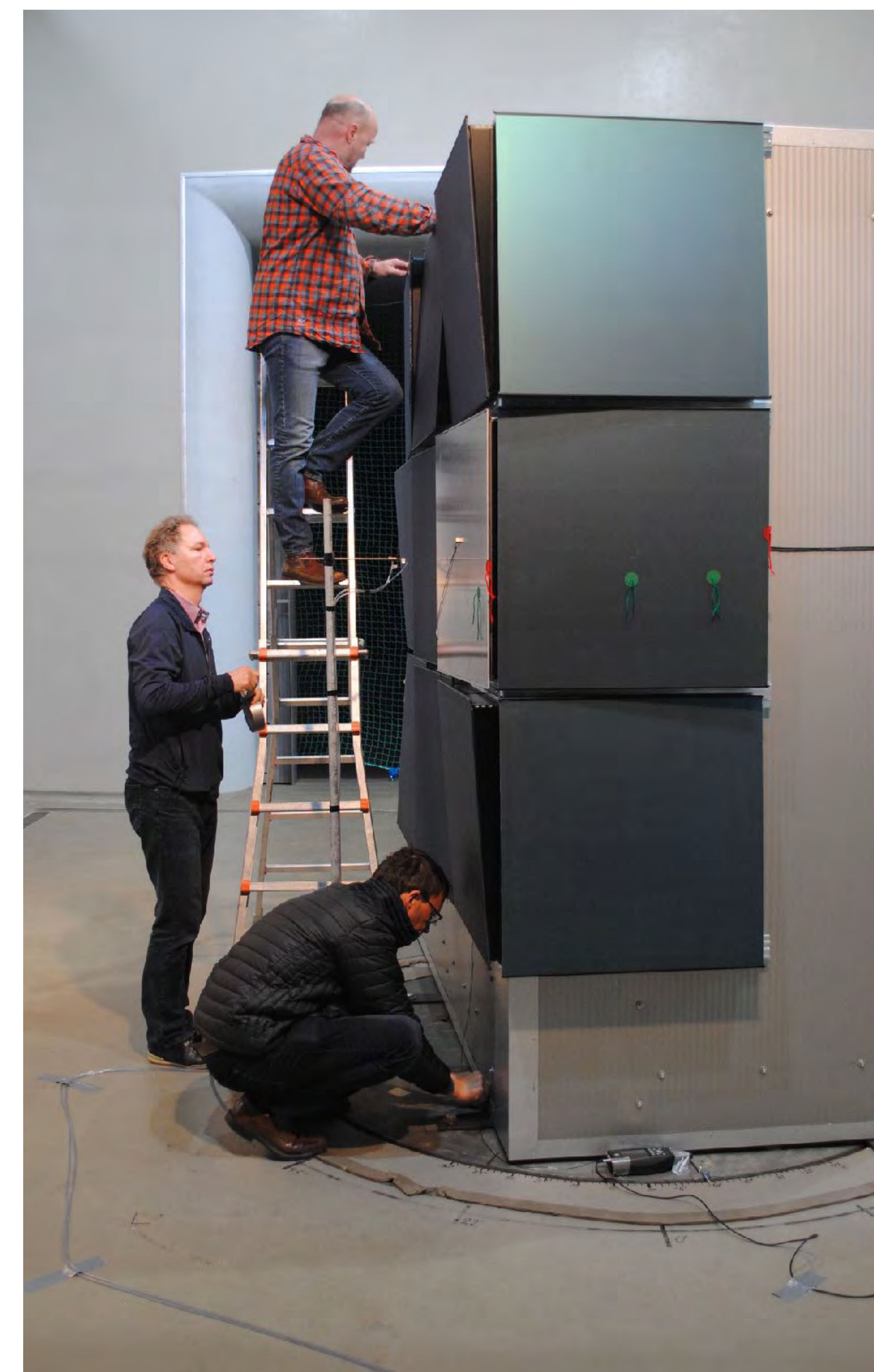
4-11. Prototype of the façade with Kingspan elements, solar modules, mounting system with brackets and rails, silicon joints, was built for tests.
