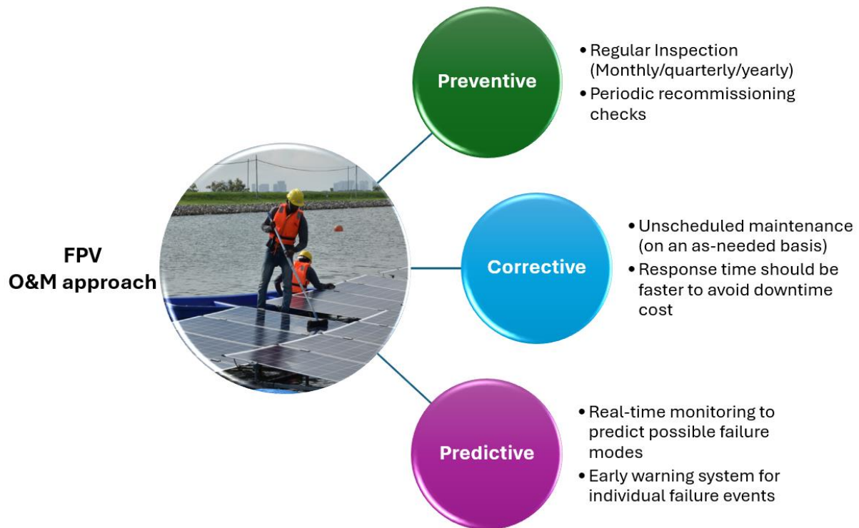
Figure 17. O&M approach for PV systems [7].
