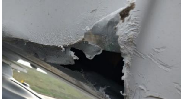
b) Rubbing and stress damage on an HDPE part
