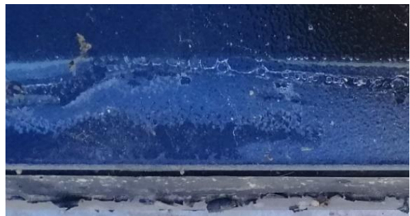
h) Partly delaminated edge seal [77]
