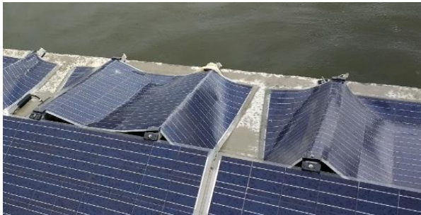
e) Damage on PV modules due to wave slamming
