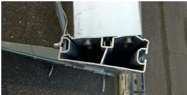
c) Torsion damage on an aluminium part
