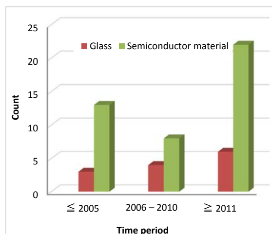
Fig. 2-26 Recovered materials for compound PV module recycling by time period
